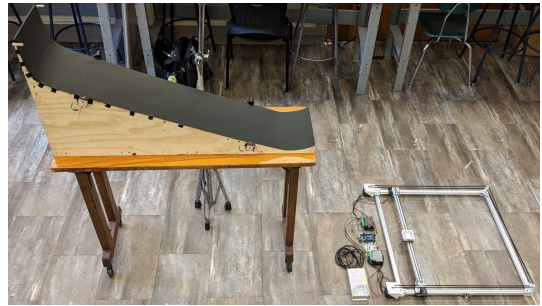
Fig. 5. Real world implementation of the environment. The ramp is made out of plywood and the robot is a 2D gantry robot controlled by an Arduino.
